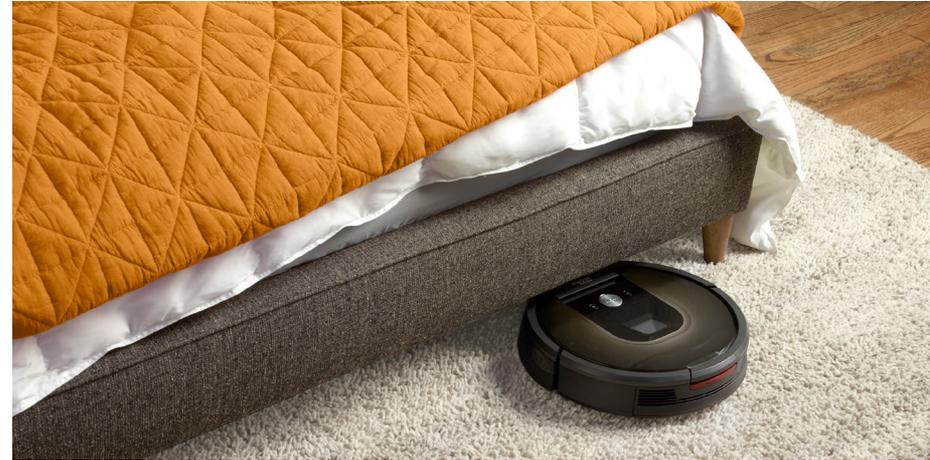
iRobot's Roomba 980 vacuuming robot uses an array of sensors to navigate an area, ensuring it cleans every part of the space it is able to reach.
