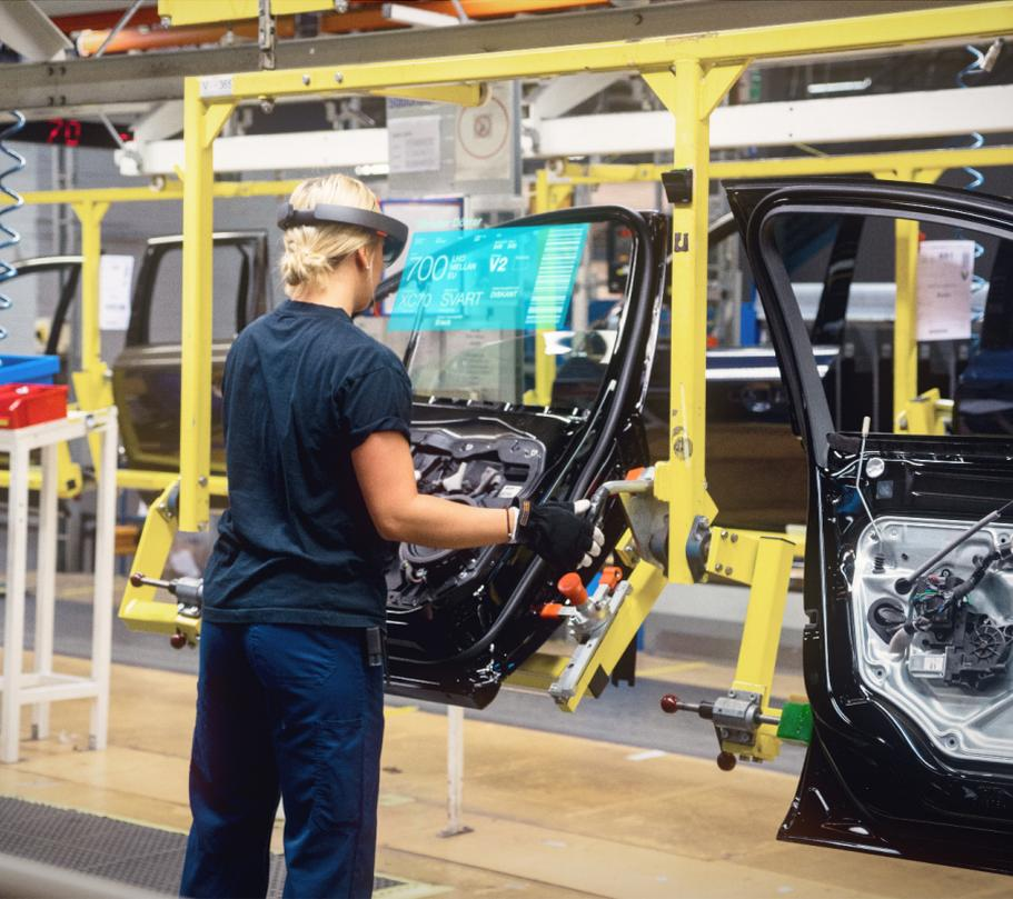
The Microsoft HoloLens allows for digital information to be overlaid onto physical reality, as seen in this manufacturing application for Volvo Cars.
