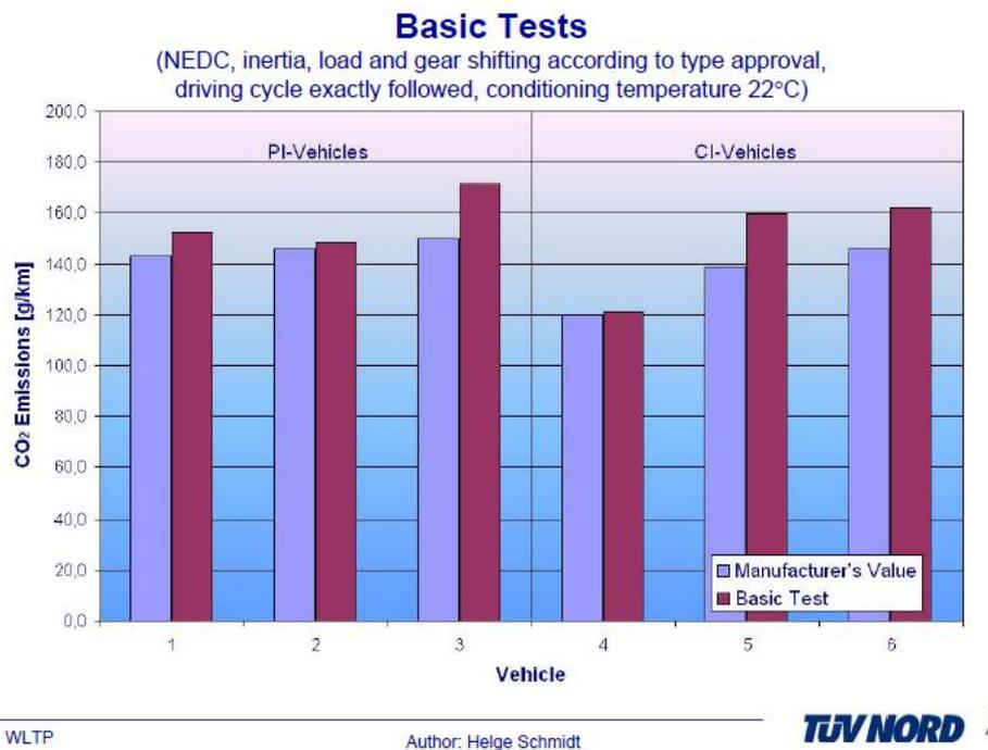
**Figure A2.2: Comparison of manufacturers’ CO<sub>2</sub> results with Schmidt and Johannsen’s own tests**
