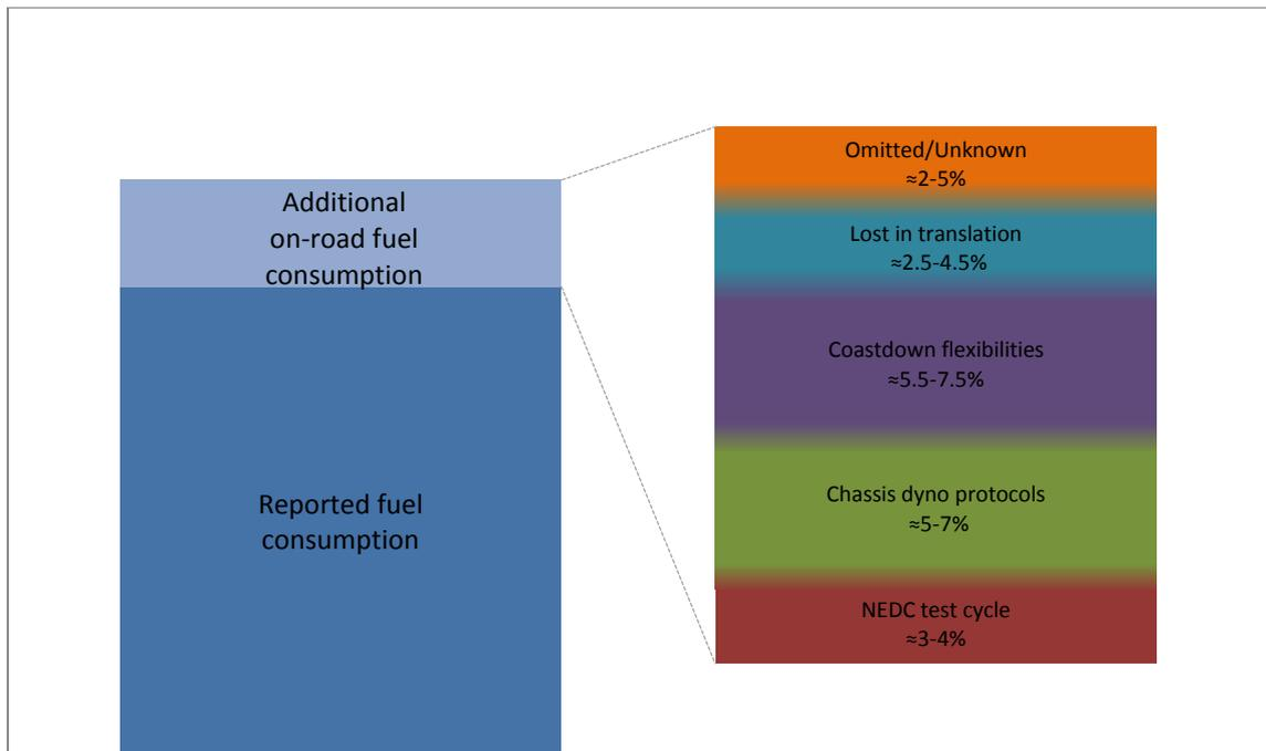
**Figure 11: Schematic of causes of the gap between official test and real-world CO<sub>2</sub> emissions**
