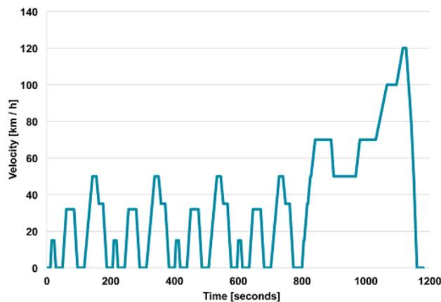
**Figure 5:** The NEDC drive cycle
