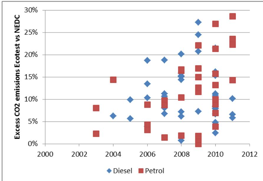
**Figure A2.3: Comparison of real-world and test data for selected car models 2003 – 11<sup>6</sup>**
