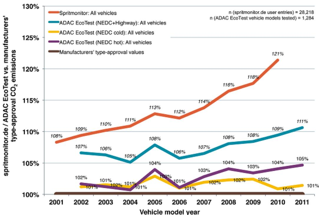
**Figure A2.4: Differences in the level of CO<sub>2</sub> emissions from other data sources as percentage of type-approval values over time**
